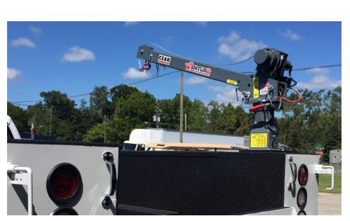
The CE6K is a 2,000 lb. crane and is available with your choice of boom sizes and mast heights to meet a variety of lifting needs. This crane features an electric 12V DC winch, manual rotation, manual extension, and manual elevation.
