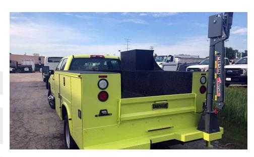
The CT2000 series cranes include the Venturo CT2003FB and CT2004FB models. The Venturo CT2003FB and CT2004FB include a heavy-duty electric winch (1.8 hp) with manual rotation, manual extension, and a folding boom.
