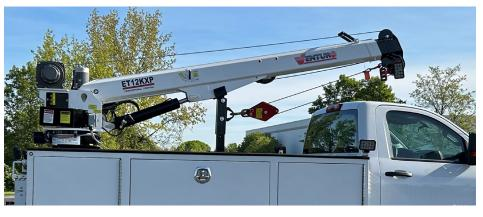
The Venturo ET12KX-15 service crane is a versatile application that is neither too large or small for a majority of lifting jobs. This crane has been utilized heavily in municipal/ public works lifting anything from service equipment to fire hydrants throughout the United States. With a 12,000 ft-lb crane rating and a 3,500 lb maximum capacity, the ET12KX-15 can be installed on trucks with a minimum 8,800 lbs GVWR.
