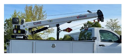
The ET12KXP-16 service crane features proportional controls, single-stage, fullhydraulic boom extension, lighter weight and easy access housing. The controls provide consistent and uninterrupted positive and ground paths with unlimited continuous rotation. The electrical components are designed for long-lasting performance, and the crane itself is the right size for the majority of lifting jobs, making it ideal for the municipal/public works sector.
