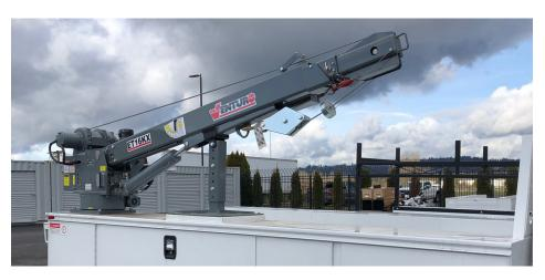
The Venturo ET16KX is a 16,000 ft-lb electric-hydraulic service crane with a 4,000 lb maximum capacity. This crane allows operators a crane application without the need for a heavy crane service body. A reinforced crane compartment on a standard utility body provides operators the strength they need on a standard service truck.
