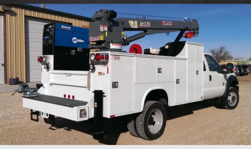
MAX. CAPACITY 6,000 LBS CRANE RATING 36,000 FT-LBS
