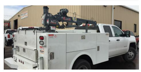
The ET6K service crane is a light-weight, cost-effective choice for a variety of industries and general service applications on any truck with a GVWR of 8,000 lbs or less. The ET6K features 2,000 lbs of maximum capacity and a 6,000 ft-lb crane rating.
