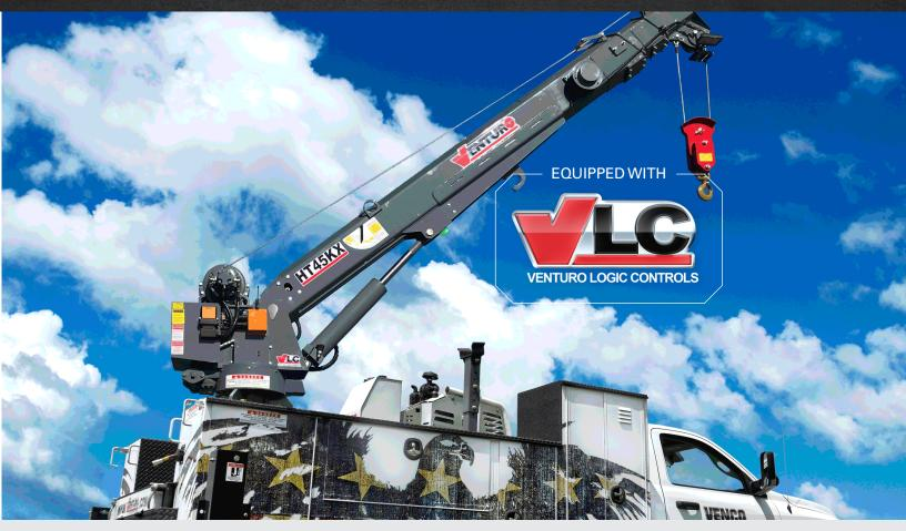
MAX. CAPACITY 7,500 LBS CRANE RATING 45,600 FT-LBS
