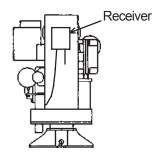
The **HT40/50KX** model without "In-Compartment Controls" requires the radio to be mounted on the right side of the crane's rear cover with the cable and antenna facing downward as shown.
