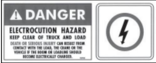
▲ SIGN NO. 15393A DISPLAYS THE INTERNATIONAL SYMBOL FOR ELECTRICITY AND WARNS OF DANGER FROM AN ELECTRICALLY CHARGED VEHICLE, CRANE, OR LOAD. FOUR ARE RECOMMENDED (ONE FOR EACH SIDE AND ONE FOR EACH END OF VEHICLE) TO BE APPLIED IN LOCATIONS WHICH ARE READILY VISIBLE TO GROUND PERSONNEL.
