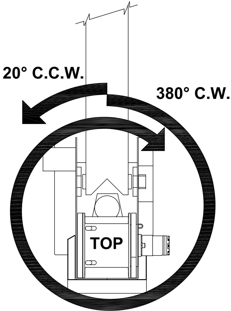
**This Venturo crane is shipped with the rotation orientation as shown above. To change the orientation rotate crane base prior to mounting to suit your application.**
