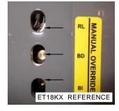
Each valve station incorporates [2] hydraulic ports and [2] coils. Manual override shafts are located in the center of the coils (see figure 1). Manual override decals are placed on each crane near the valve assembly. These decals provide a visual aid that helps the operator determine the function designations (Reference figure 2).
