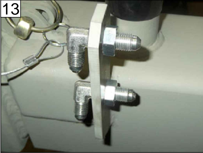
FASTEN BULKHEAD FITTINGS, EACH SIDE PAGE 19 - ITEM 9
