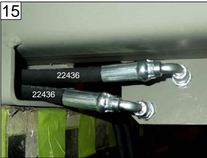
INSTALL HOSES, ROUTE THROUGH UNDERCARRIAGE PAGE 19 - ITEM 10
