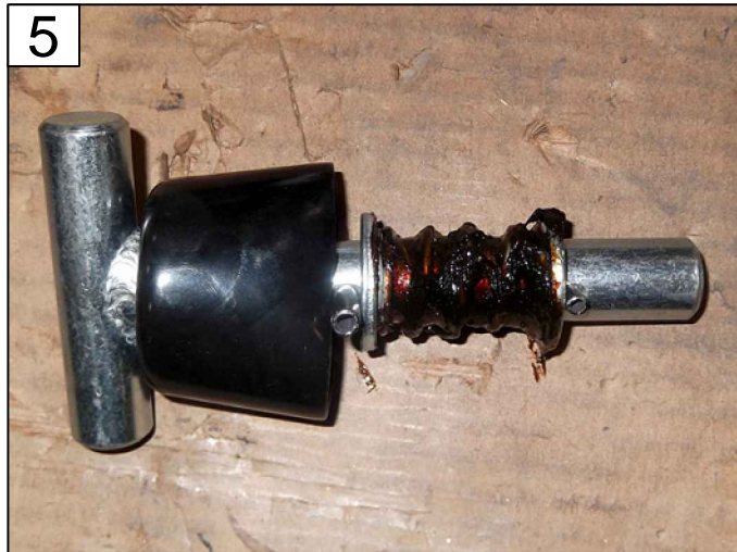
GREASE BOTH LOCK PINS' SPRINGS PAGE 17 - ITEM 4
