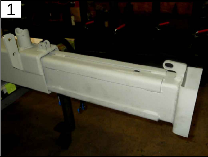
SLIDE LONG, RIGHT-SIDE PULLOUT INTO CROSSTUBE PAGE 17 - ITEM 1
