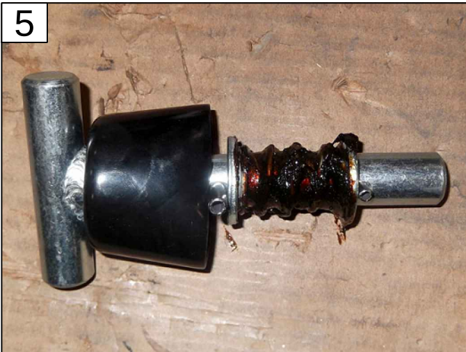
GREASE BOTH LOCK PIN'S SPRINGS PAGE 17 - ITEM 4
