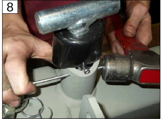
GUIDE ROLL PINS UNTIL FLUSH ON BOTH ENDS
