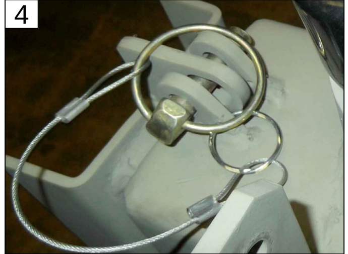
ENSURE PIN IS THROUGH ALL TABS & CLAMP MEETS END REPEAT STEPS 3 & 4 FOR OPPOSITE END
