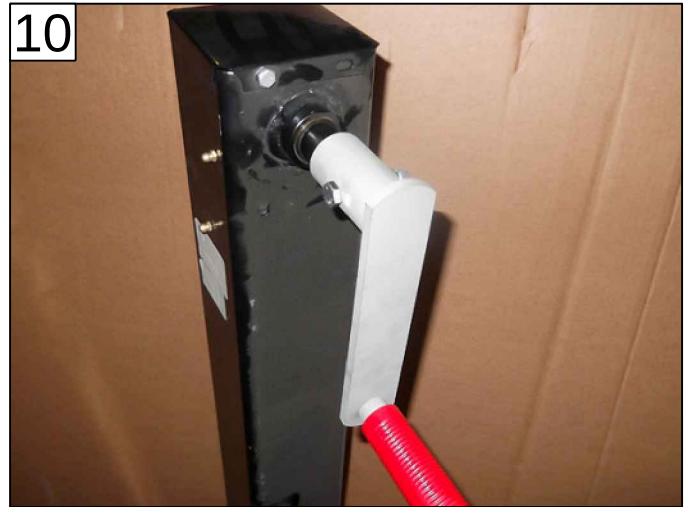
FOR 24962-CD, FASTEN CRANK-HANDLE TO LEG SHAFT ▲ PAGE 17 - ITEMS 8, 9, 10, 11, & 12
