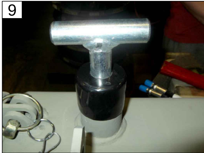
COVER WITH RUBBER BOOT REPEAT STEPS 5 TO 9 FOR OPPOSITE END
