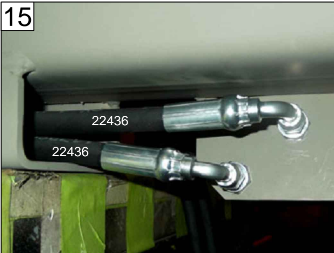
INSTALL HOSES, ROUTE THROUGH UNDERCARRIAGE PAGE 19 - ITEM 10
