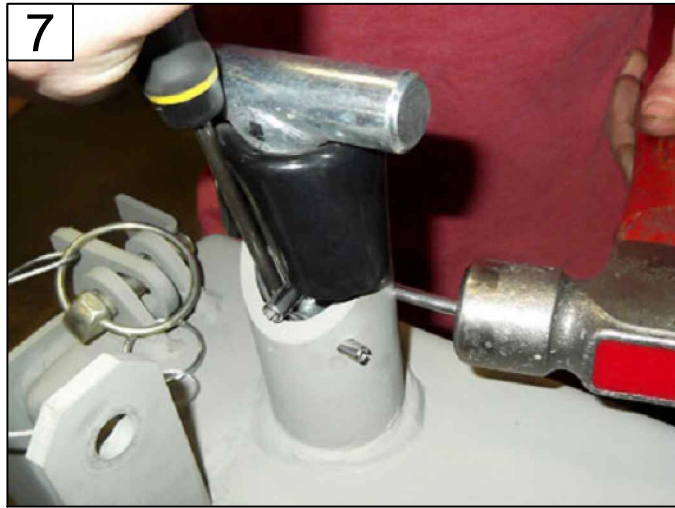
PUSH SPRING-LOADED WASHER DOWN START DRIVING ROLL PINS THROUGH
