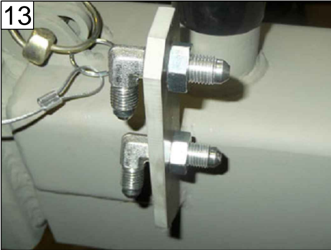
FASTEN BULKHEAD FITTINGS, EACH SIDE PAGE 19 - ITEM 9
