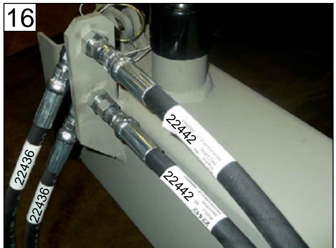
INSTALL HOSES, REFER TO 'HYDRAULIC MAPPING' PAGE 19 - ITEMS 10 & 13
