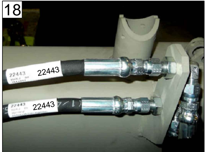
INSTALL HOSES, REFER TO 'HYDRAULIC MAPPING' PAGE 19 - ITEM 14
