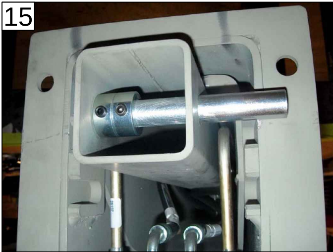
INSERT SHAFT & COLLARS INTO CYLINDER HOUSING
