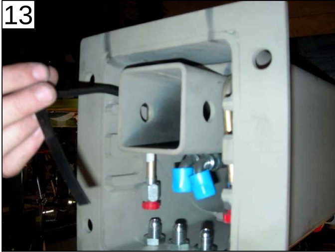
UNTIE PULLOUT CYLINDER HOUSING & PLUMBING
