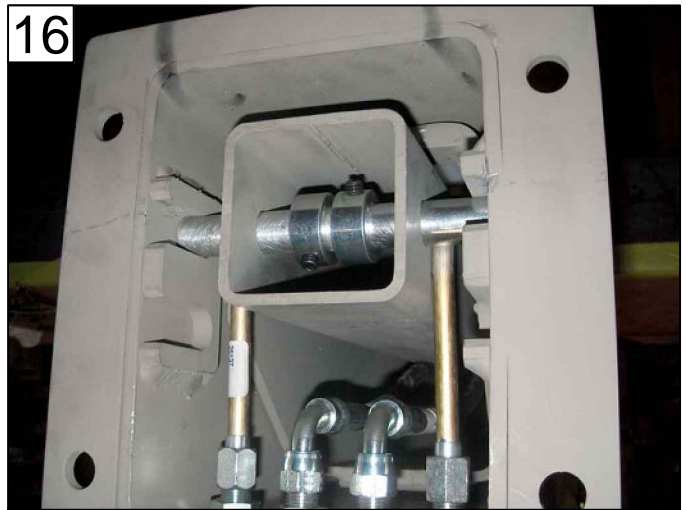
PUSH SHAFT INTO TOP SLOT OF CROSSTUBE
