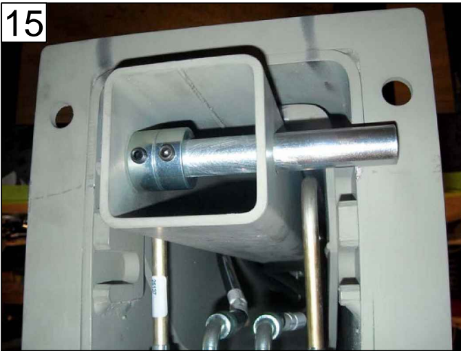
INSERT SHAFT & COLLARS INTO CYLINDER HOUSING
