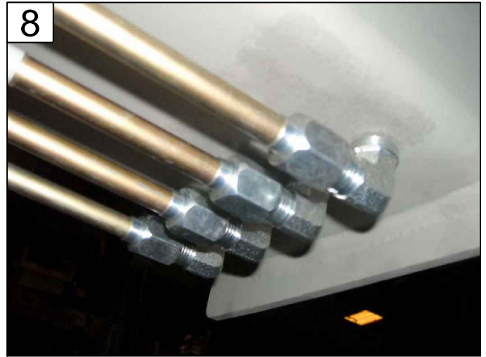
FASTEN 25138 TUBES TO BULKHEADS PAGE 15 - ITEM 13
