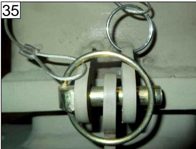
35 ENSURE PIN IS THROUGH ALL TABS & CLAMP MEETS END
