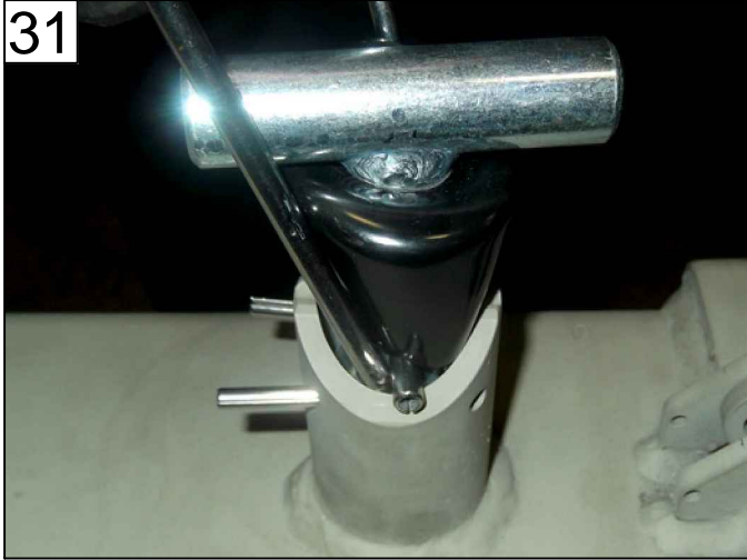
31 PLACE T-HANDLE PUSH SPRING-LOADED WASHER DOWN
