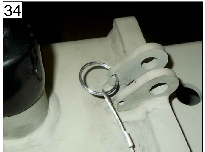
34 ATTACH SECURITY PIN'S KEY-RING ON EITHER TAB PAGE 21 - ITEM 12
