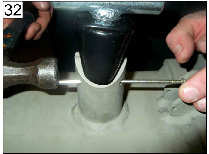
32 DRIVE ROLL PINS THROUGH FLUSH ON BOTH ENDS
