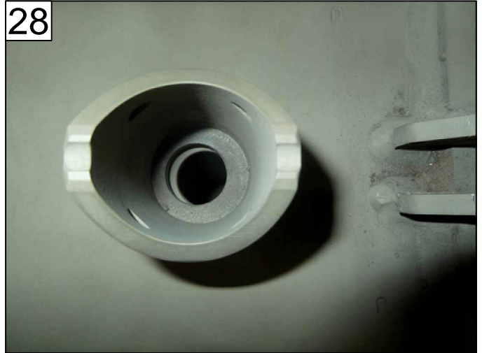
LINE UP LOCK-PIN HOLES FOR PULLOUT & CROSSTUBE
