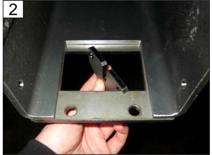
REFERENCE FOR PLACING AXLE SUPPORTS
