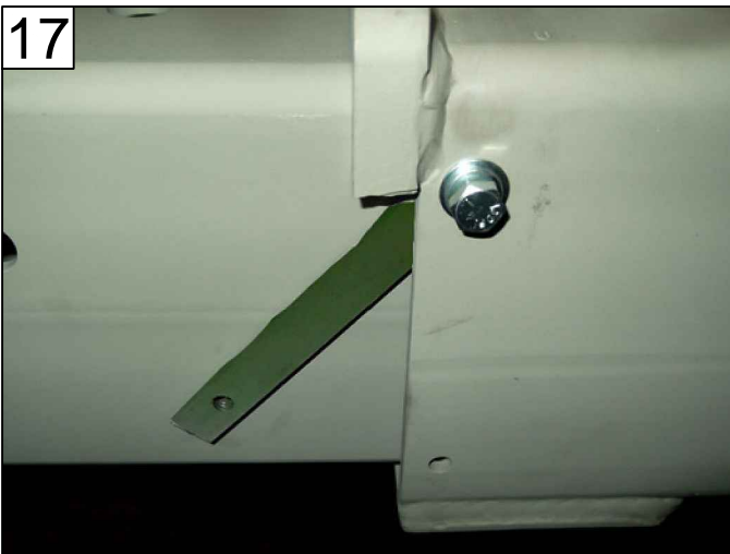
FASTEN NUT BAR RETAINERS INTO CROSSTUBE PAGE 21 - ITEMS 7, 8, & 9
