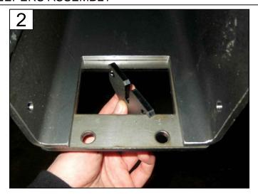
REFERENCE FOR PLACING AXLE SUPPORTS
