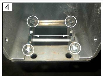
MAKE [4] TACKS ON ENDS OF SUPPORTS ENSURE AXLE ROD FITS
