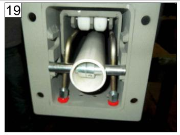
INSERT SHAFT THROUGH PIPE, LOCK COLLARS INSIDE PAGE 21 - ITEMS 14 & 15
