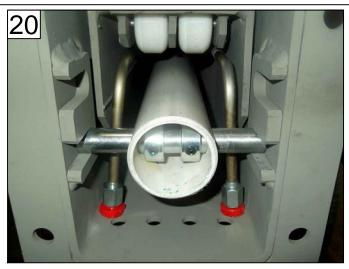
PUSH SHAFT INTO BOTTOM SLOT OF CROSSTUBE LOCTITE & FASTEN COLLARS CENTER & FLUSH
