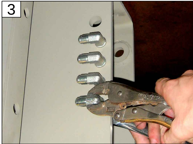
3 FASTEN BULKHEAD FITTINGS, POINTING CURB-SIDE PAGE 17 - ITEM 9
