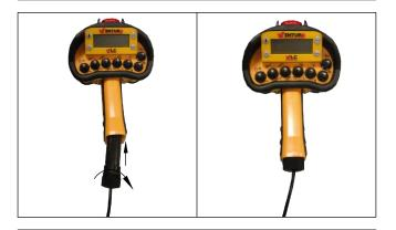
Insert end of CAN cable into Transmitter handle and tighten in place.
