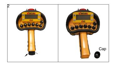
Unscrew cap from Transmitter handle, remove Transmitter battery and set aside.
