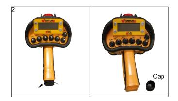
Unscrew cap from Transmitter handle, remove Transmitter battery and set aside.
