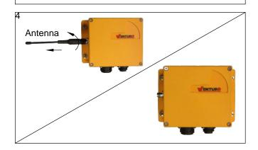
Unscrew and remove antenna from the Receiver and set aside.
