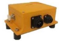
The receiver is the main processing unit and Communications Area Network (CAN) master for the system.
