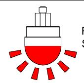
RED SOLID OVERLOAD (MAX CAPACITY) CONDITION
