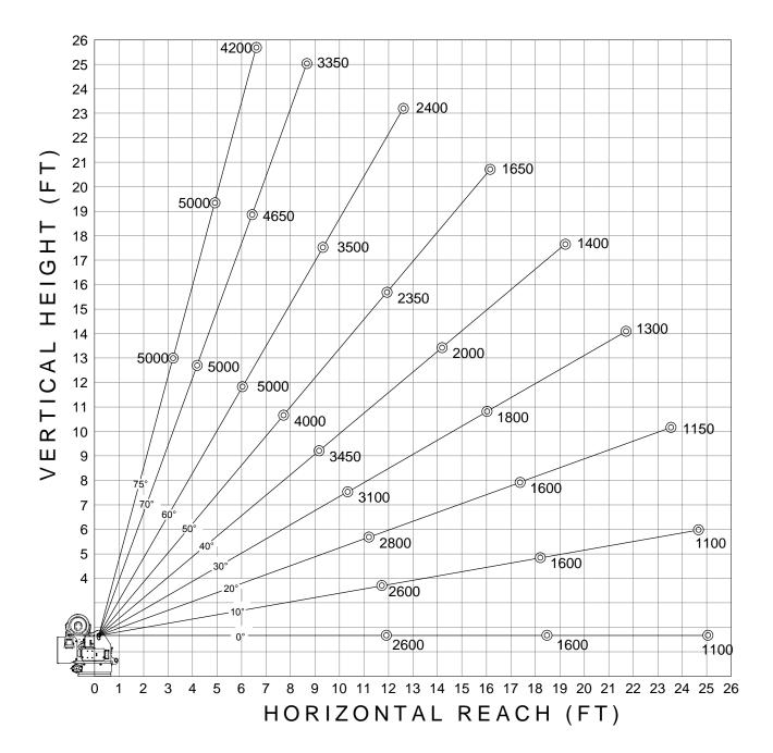
WEIGHT OF LOAD HANDLING DEVICES ARE PART OF THE LOAD AND MUST BE DEDUCTED FROM THE GROSS CAPACITY.
