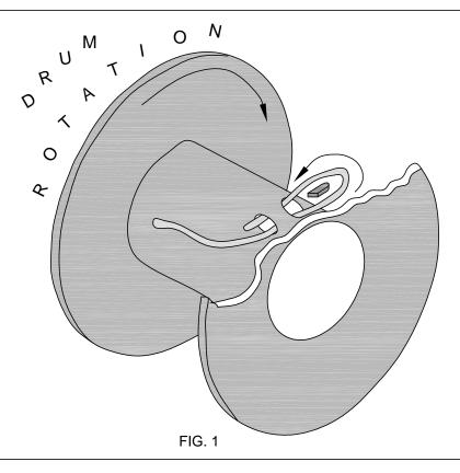
STEP 1: UNWIND COIL OF WIRE ROPE BY 'ROLLING' ALONG THE FLOOR. THIS WILL PREVENT 'KINKING'.
