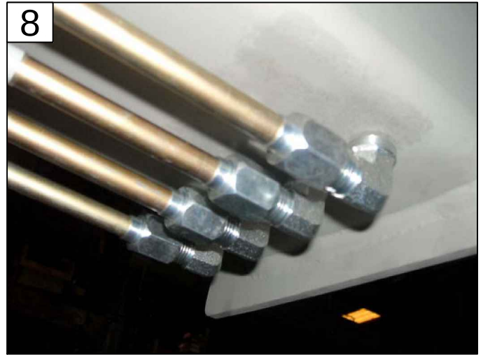
FASTEN 25138 TUBES TO BULKHEADS PAGE 15 - ITEM 13
