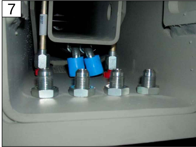
FASTEN BULKHEADS - SEE NEXT STEP'S IMAGE PAGE 15 - ITEM 12
