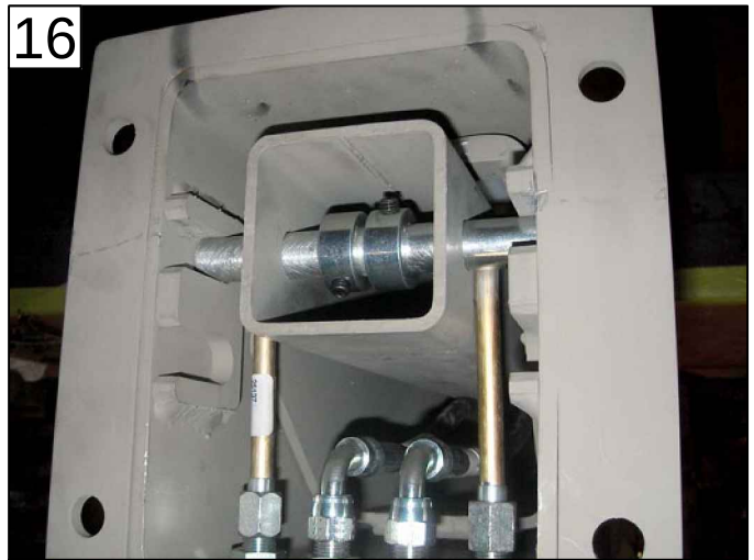
PUSH SHAFT INTO TOP SLOT OF CROSSTUBE
