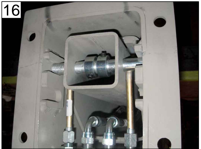
PUSH SHAFT INTO TOP SLOT OF CROSSTUBE
