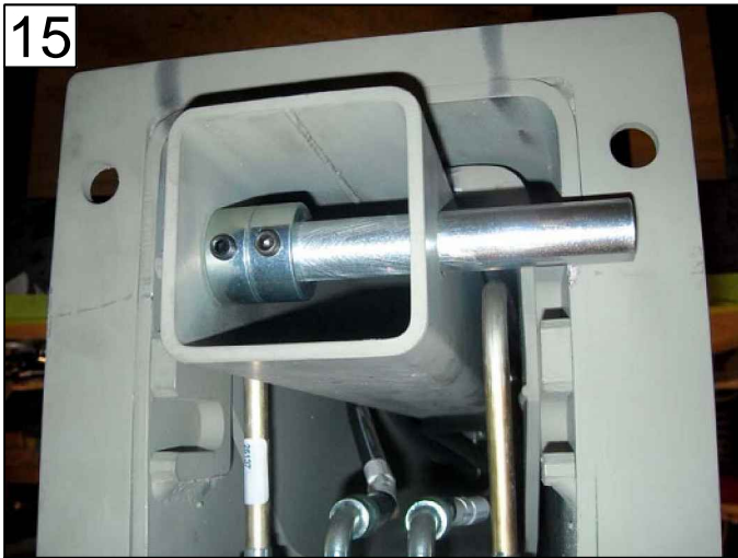
INSERT SHAFT & COLLARS INTO CYLINDER HOUSING
