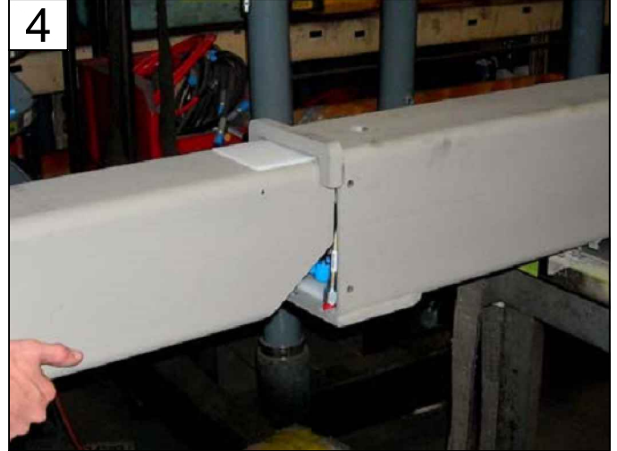
SLIDE PULLOUT INTO CROSSTUBE
