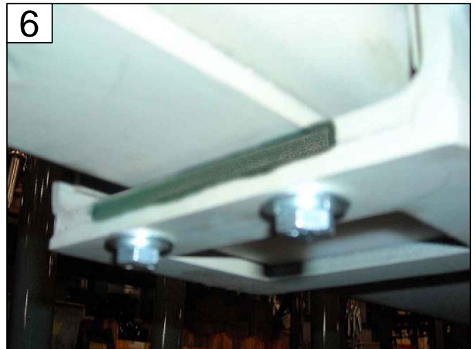
FASTEN 25077 NUT BAR RETAINER IN CROSSTUBE PAGE 15 - ITEMS 3, 4, 5, & 6
