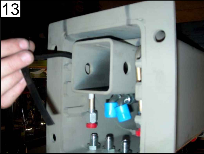
UNTIE PULLOUT CYLINDER HOUSING & PLUMBING
