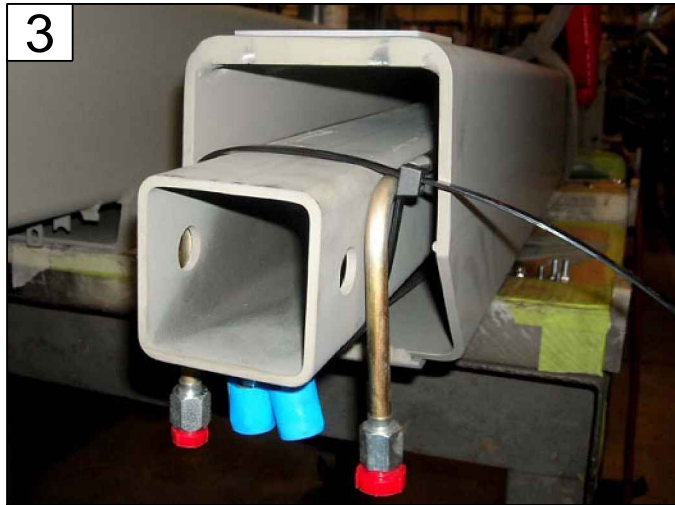
ENSURE PULLOUT CYLINDER HOUSING & PLUMBING ARE TIED
