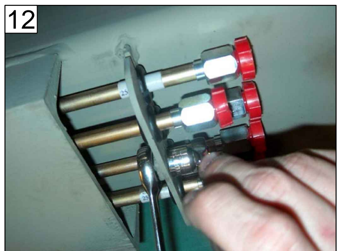
FASTEN CLAMP, PAGE 15 - ITEMS 4 & 17 REPEAT STEPS 9 TO 11 FOR OPPOSITE CLAMP
