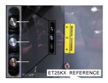
Each valve station incorporates [2] hydraulic ports and [2] coils. Manual override shafts are located in the center of the coils (see figure 1). Manual override decals are placed on each crane near the valve assembly. These decals provide a visual aid that helps the operator determine the function designations (Reference figure 2).
