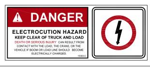
SIGN NO. 15393 DISPLAYS THE INTERNATIONAL SYMBOL FOR ELECTRICITY AND WARNS OF DANGER FROM AN ELECTRICALLY CHARGED VEHICLE, CRANE, OR LOAD. FOUR ARE RECOMMENDED (ONE FOR EACH SIDE AND ONE FOR EACH END OF VEHICLE) TO BE APPLIED IN LOCATIONS WHICH ARE READILY VISIBLE TO GROUND PERSONNEL.
