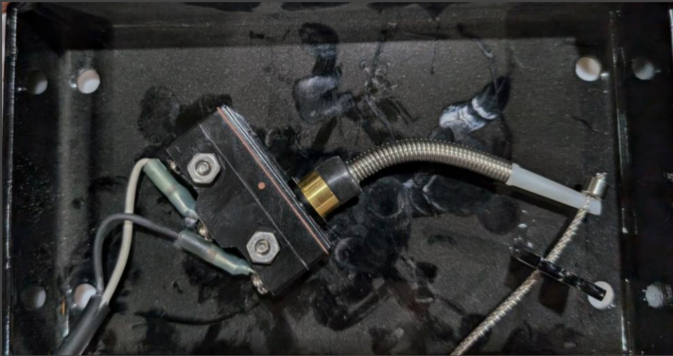
Normal operation: Tension on wire connected to wand switch and wand switch actuated
