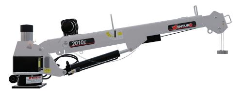
The 2010E service crane is a light-weight, cost-effective choice for a variety of industries and general service applications on any truck with a GVWR of 8,000 lbs or less. The 2010E features 2,000 lbs of maximum capacity and a 6,000 ft-lb crane rating.
