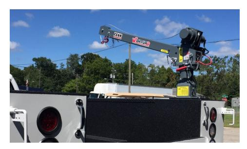
The CE6K is a 2,000 lb. crane and is available with your choice of boom sizes and mast heights to meet a variety of lifting needs. This crane features an electric 12V DC winch, manual rotation, manual extension, and manual elevation.
