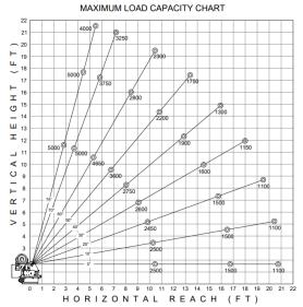
WEIGHT OF LOAD HANDLING DEVICES ARE PART OF THE LOAD AND MUST BE DEDUCTED FROM THE GROSS CAPACITY.
