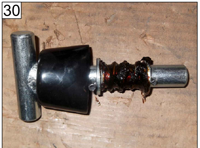
GREASE T-HANDLE'S SPRING REFERENCE 25461-1 ITEM 11
