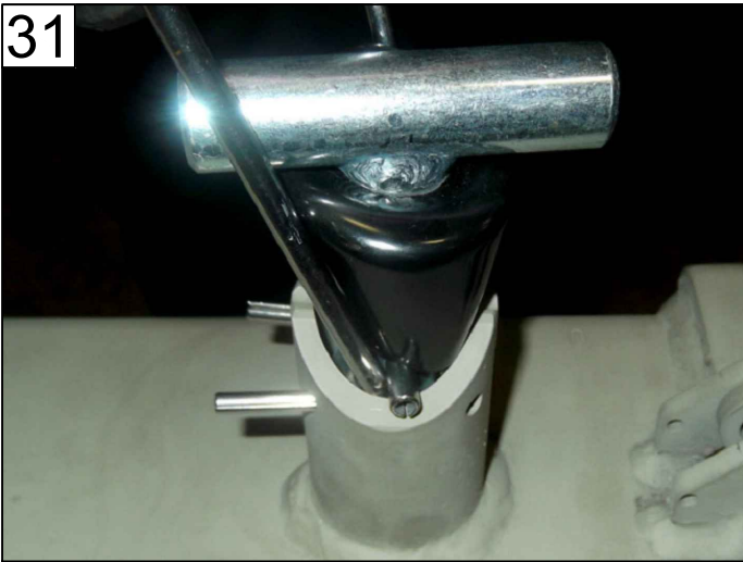
PLACE T-HANDLE PUSH SPRING-LOADED WASHER DOWN
