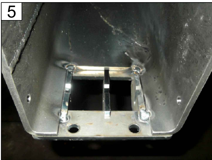
PLACE LAST AXLE SUPPORT CENTERED
