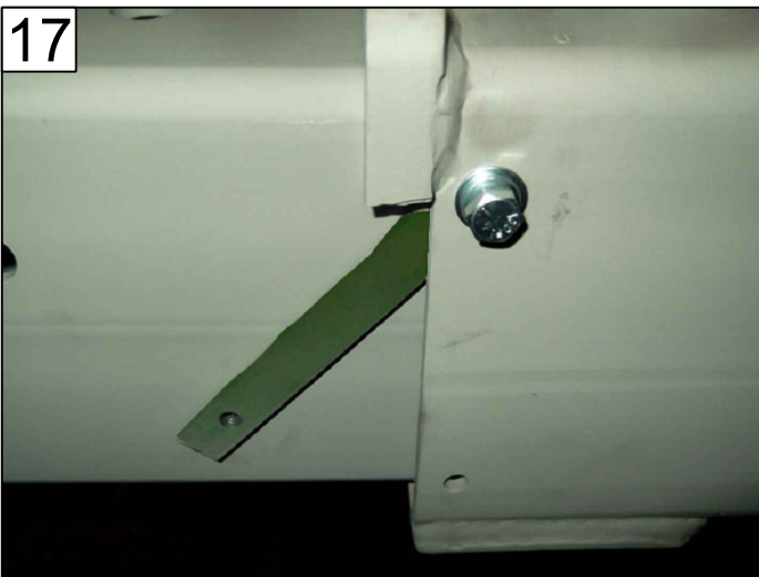
FASTEN NUT BAR RETAINERS INTO CROSSTUBE 25461-1, ITEMS 6, 7, & 8
