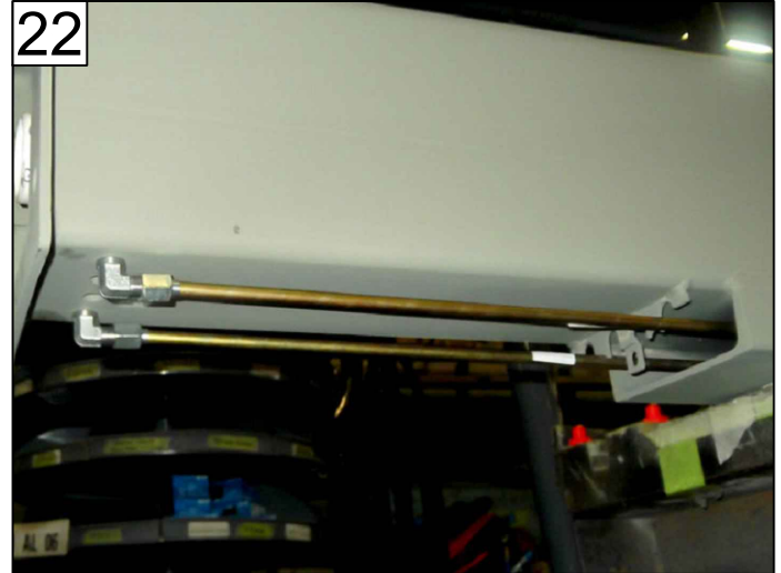
22 FASTEN 60" HYDRAULIC TUBES TO BULKHEADS REFERENCE 25461-1 ITEM 23
