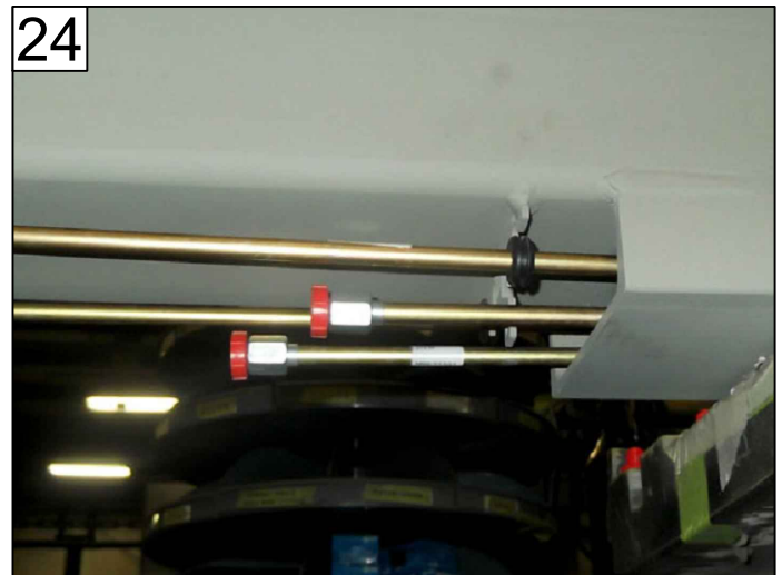
24 PLACE 47" HYDRAULIC TUBES REFERENCE 25461-1 ITEM 24
