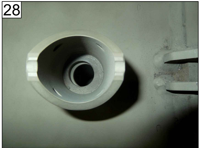
LINE UP LOCK-PIN HOLES FOR PULLOUT & CROSSTUBE
