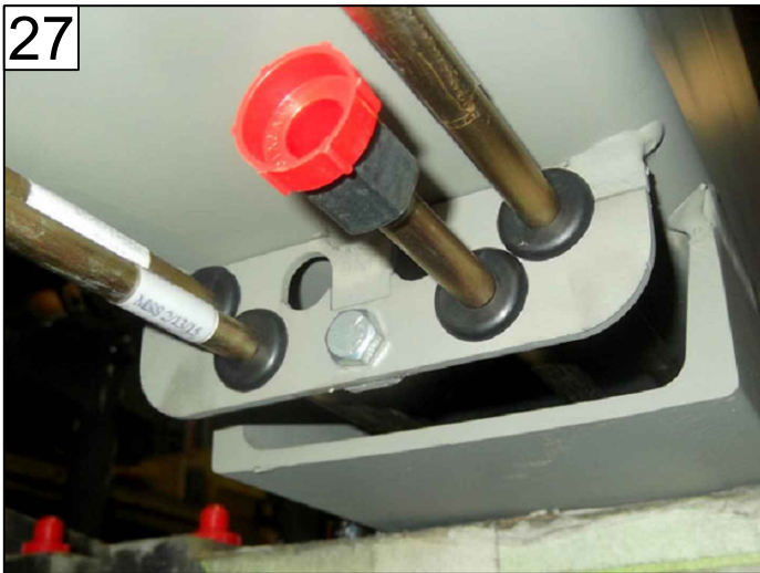
FASTEN CLAMP, ITEMS 27 & 28 REPEAT STEPS 25 TO 27 FOR OPPOSITE CLAMP
