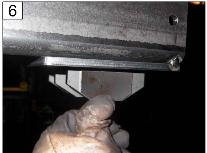
PLACE EACH AXLE KEEPER ON OUTSIDE OF SUPPORTS FLUSH WITH EDGES EVEN
