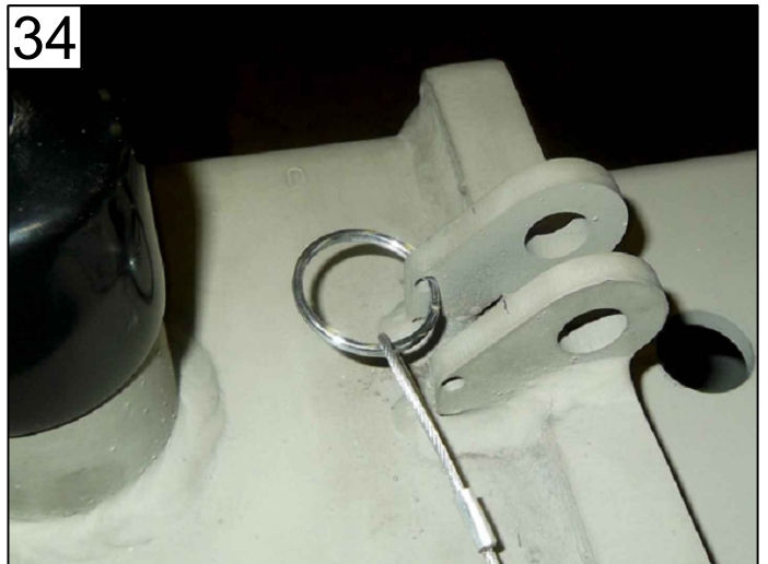
ATTACH SECURITY PIN'S KEY-RING ON EITHER TAB REFERENCE 25461-1 ITEM 12
