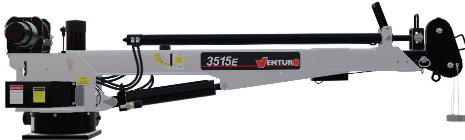
The Venturo 3515E service crane is a versatile application that is neither too large or small for a majority of lifting jobs. This crane has been utilized heavily in municipal/public works lifting anything from service equipment to fire hydrants throughout the United States. With a 12,000 ft-lb crane rating and a 3,500 lb maximum capacity, the 3515E can be installed on trucks with a minimum 8,800 lbs GVWR.
