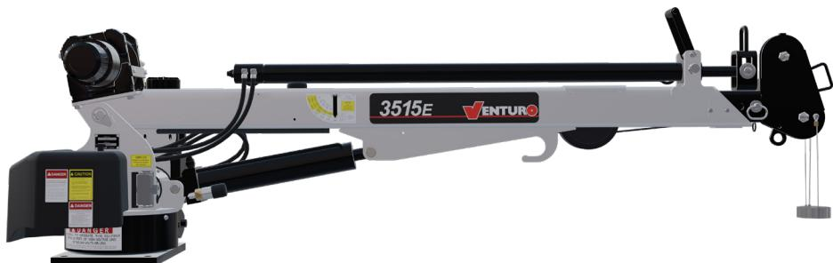
The Venturo 3515E service crane is a versatile application that is neither too large or small for a majority of lifting jobs. This crane has been utilized heavily in municipal/public works lifting anything from service equipment to fire hydrants throughout the United States. With a 12,000 ft-lb crane rating and a 3,500 lb maximum capacity, the 3515E can be installed on trucks with a minimum 8,800 lbs GVWR.
