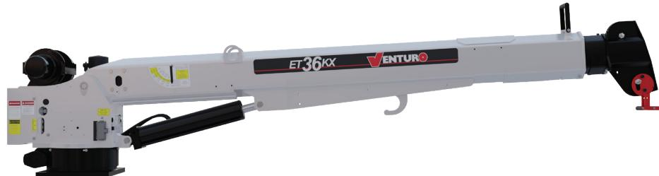
The Venturo ET36KX is a 36,000 ft-lb electric-hydraulic service crane with a 6,000 lb maximum capacity at 6 ft. This larger crane gives operators the distance and strength they need for heavier loads at a short distance. This electric crane features full-hydraulic boom extension out to 20 ft.
