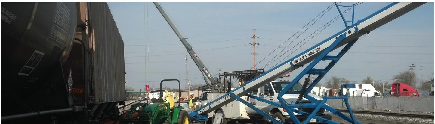
"The ET36KX from Venco Venturo was a great solution for our situation because it meant we didn't have to have any manual pull out and it could extend all the way to 20 feet hydraulically," Zurliene said. "Although we didn't necessarily need the weight capacity, we needed the height capacity for our service truck to reach farther with the truck crane in some instances in order to avoid needing to have an outside truck come in to meet our needs."
